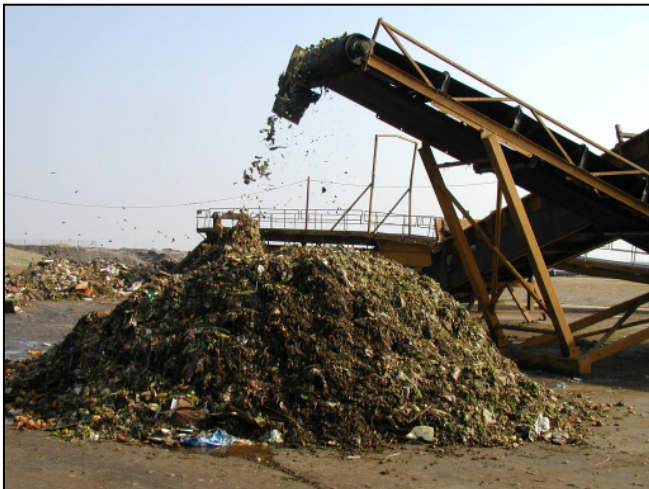
Organic matter is sorted at Jepson Prairie Organics prior to being placed in windrows to begin the composting process.
