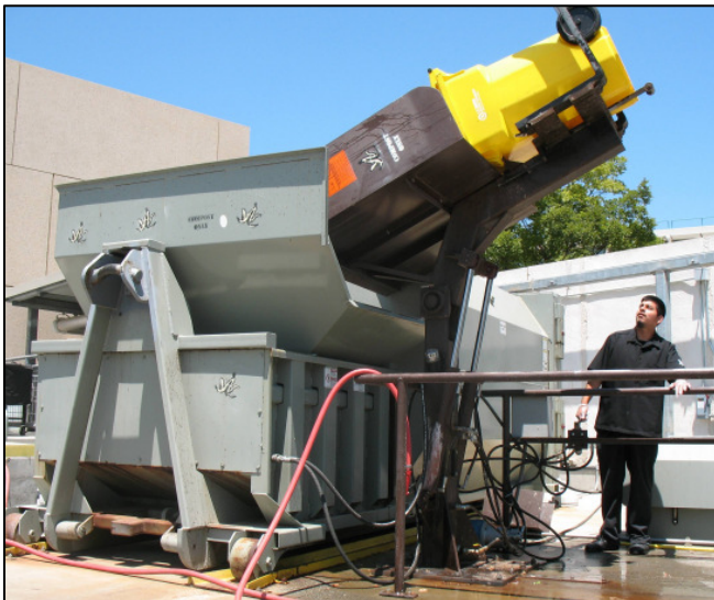
Segundo Dining Room has a specially designed and dedicated compost compactor to facilitate the collection and staging needs of compost-ready material from both the dining room and ancillary dining units across campus. When full, the compactor is loaded onto a flatbed truck and hauled to Jepson Prairie Organics.
